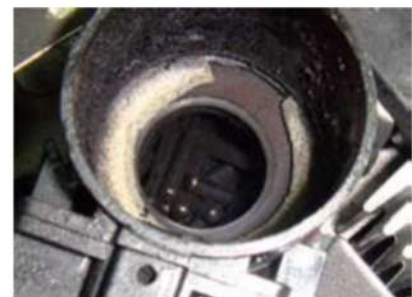
Collapsed OE needle bearing after critical speed durability test
