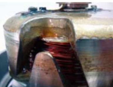
Inferior varnish process on O.E. alternator causes noisy operation & interference between internal stator & rotor components.
